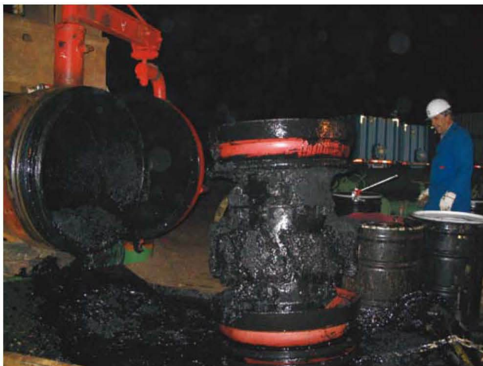
Figure 1. Black powder from a natural gas pipeline.
