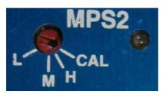
Once the sensor has finished its calibration, the LED will begin double blinking every 2 seconds. This indicates successful calibration.
